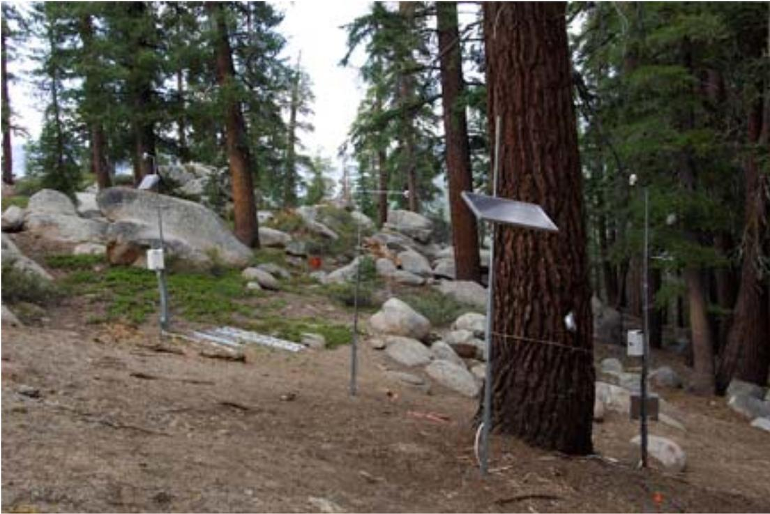
**Figure 18.** Acoustic snow-depth sensors under canopy, drip edge and in the open, Wolverton site 3, high elevation, south facing. A set of soil moisture sensors are located beneath each snow sensor. Additional snow sensors that are part of the instrument node are deployed within 50 m.
