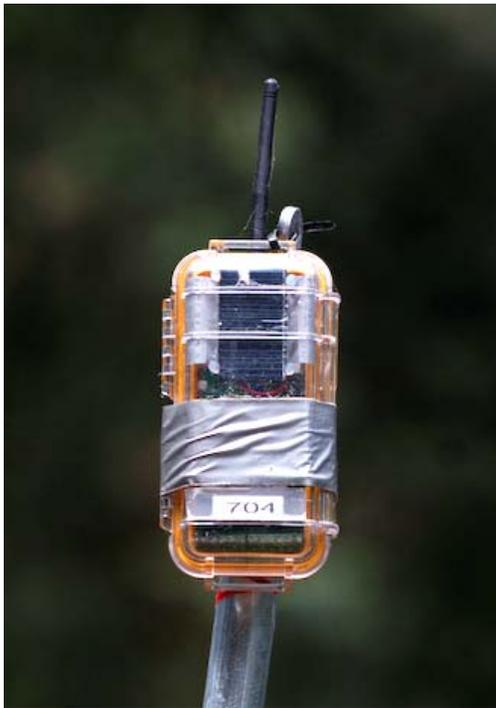
**Figure 10. Crossbow prototype atop 10-m pole at Wolverton, for telemetering soil matric potential data.**
