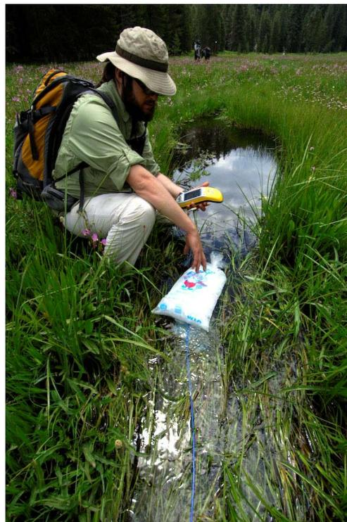
**Figure 14. Calibration of DTS cable with ice, Long Meadow.**
