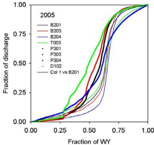
**Figure 4. Cumulative streamflow for 8 KREW catchments, illustrating the transition from rain (D102) to snowmelt (B204) dominance.**
