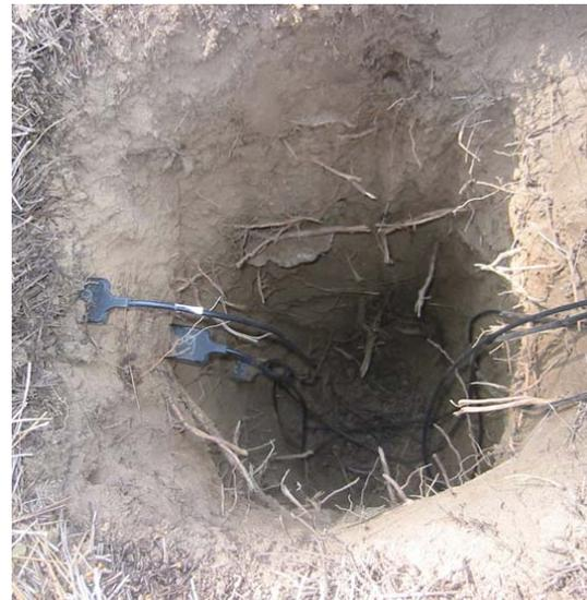
**Figure 12. Placement of Decagon soil moisture probes at 10-, 30-, 60- and 90-cm depths.**
