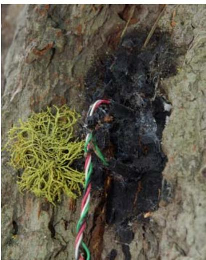
**Figure 17. Wolverton sap flow sensor.**
