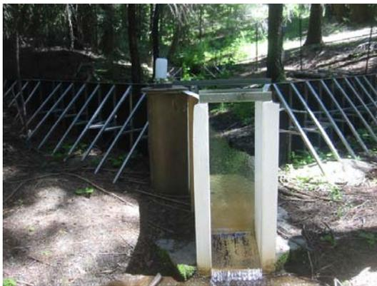
**Figure 6. KREW stream gage. Each stream has 2-stage flumes, for both high and low flows.**
