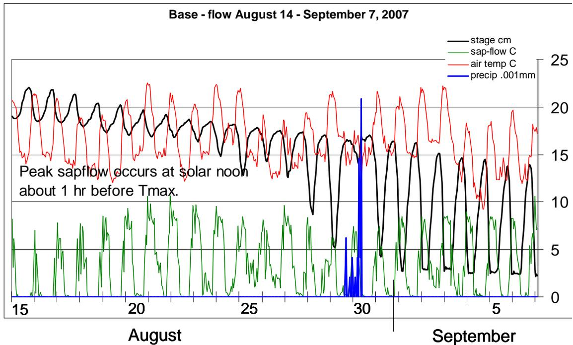
**Figure 3.** Wolverton Creek stage, precipitation, air temperature and sap flow data for a baseflow period, 2007, illustrating the value of high-frequency, coincident data. Note tracking of air temperature and sap flow, and diel stream stage response to evapotranspiration. After precipitation event, the increase in evapotranspiration is thought to be due to understory and riparian vegetation, as trees showed no response.
