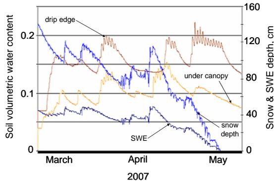
**Figure 16. Soil moisture and snowpack data from instrument cluster illustrating how rain-snow transition zone undergoes rapid seasonal changes, going from snowcover to wet soil to dry soil over 1-2 months. Note diel fluctuations in soil moisture during snowmelt and also wetter soil at canopy dip edge versus under canopy.**
