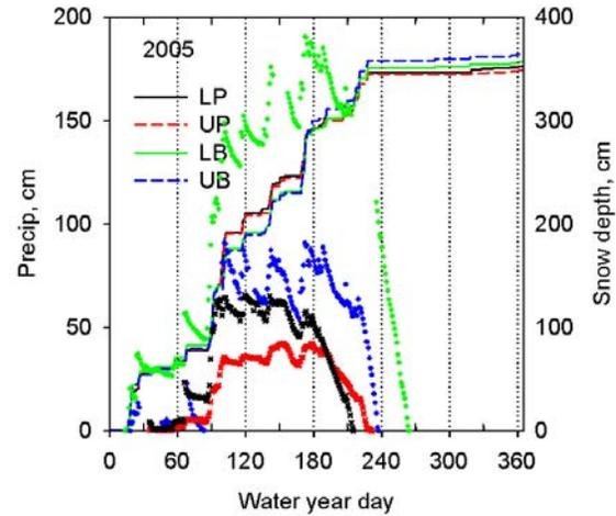
**Figure 5. Snow depth shown with cumulative precipitation for 2005, illustrating the differing lags between the two across the higher (UB) versus lower (LP) sites. Note coincidence of precipitation versus lags in snowmelt between the sites.**
