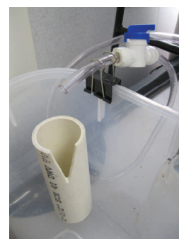
Fig 5. Valve attached to side of tub
