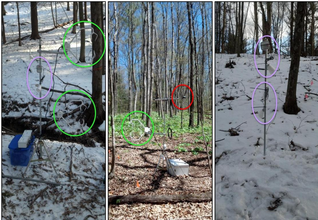
**Figure 2-4.** Three example instrument stations at Shale Hills. Instruments are circled in red (net radiometer), green (sonic anemometer), and purple (logger/temperature sensor). Stations pictured are representative of all surface measurement sites.
