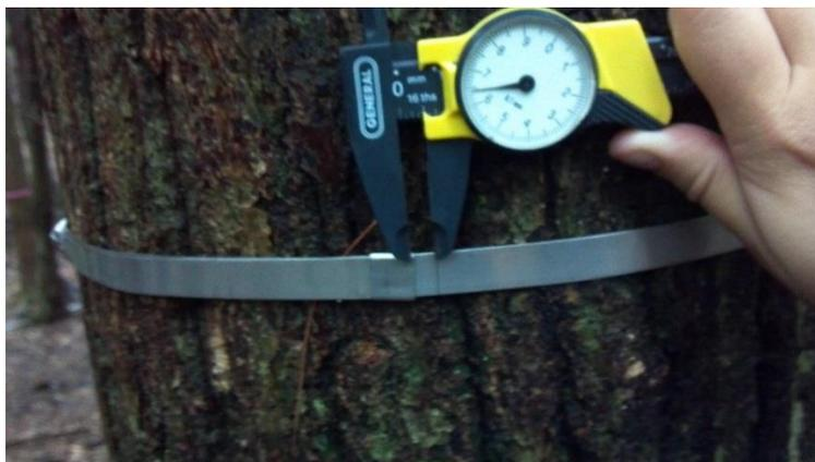
Figure 1.3. A dendroband constructed at the Susquehanna Shale Hills Critical Zone Observatory. Constructed out of a metal band, metal spring, and metal loop to measure radial growth.
