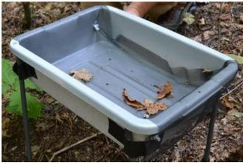
Figure 1.1. A sample litter trap from the Susquehanna Shale Hills Critical Zone Observatory. The traps were made using a plastic tub (0.1518 m<sup>2</sup> area, 33 x 46 x 12cm), suspended net, and plastic rods to stabilize the trap 0.5 meters off of the ground.
