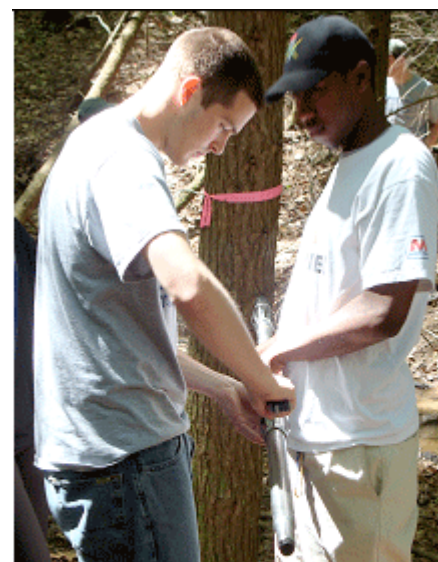
Figure 2b) One of many logging tool, the optical televiewer. Nate Wysocki (PSU undergrad) and Maurice Dukes (Fort Valley State undergrad) control operation.
