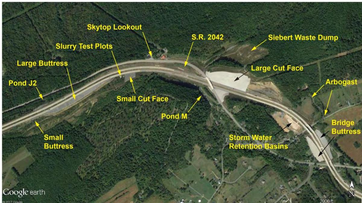
**Figure 8. Google Earth view of Skytop showing important sites, including GeoWeb installations (light gray areas).**
