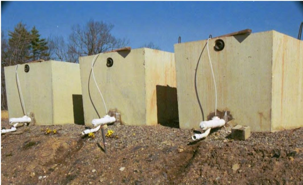
**Figure 11.** *Septic tanks with white sampling valve and a small, near vertical plastic tube that serves as a manometer to indicate water level in each tank. Additives tested were Bauxsol™ in the right tank, MgO in the center tank and limestone in the left tank (from Barnes and Gold, 2008).*
