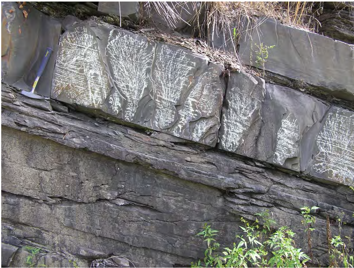
Figure 6-1. Joints in interbedded siltstone of the Brallier Formation in a road cut along Penn Street off Route 22 in Huntingdon, PA. Multiple en-echelon cracks propagate upward into a siltstone layer from a shale-siltstone interface with a J_2 joint in shale acting as the parent.
