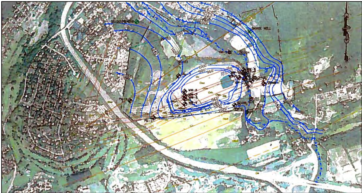
Figure H6-5. Geology and water table for the Oak Hall Quarry Area.
