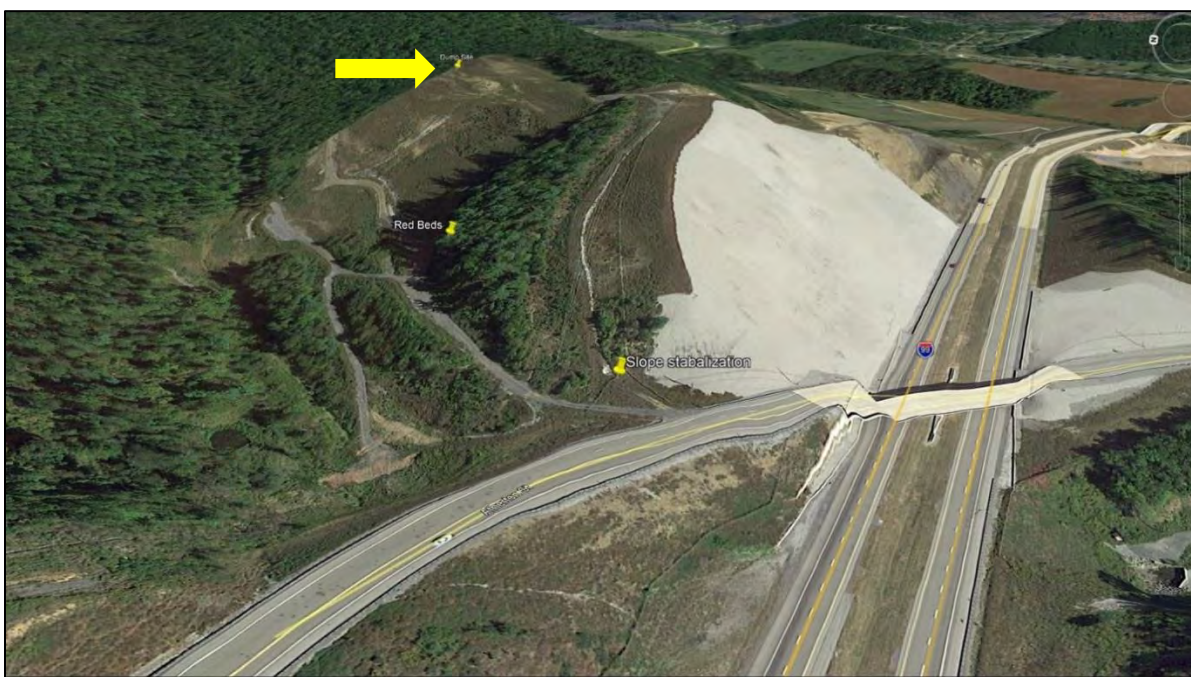
Figure E7-1. View looking east of Skytop and the Siebert Dump site on the north slope. The sulfide veins on the slope have been covered with geotextiles. Material from this pyrite-veined road cut was used as fill for the buttress and elevated road bed. Areas of interest (Siebert dump, Juniata redbeds, slope stabilization) are marked by the yellow “push” pins. The yellow arrow points to the Siebert dump.
