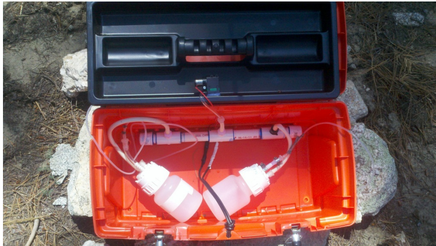
Figure 4. New battery operated pump system for Prenart sampling developed by Nate Abramson (SCM-CZO field scientist) has significantly improved pore water sample recoveries from the vadose zone.
