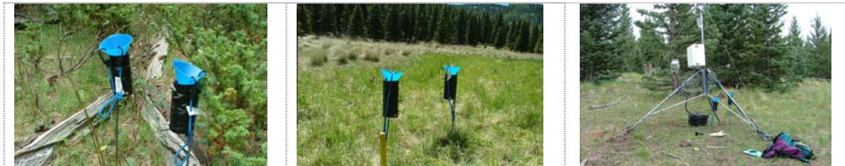
Figure 11. Bulk rain collectors: a) La Jara flume, b) Upper Jaramillo flume, c) ZOB meteorological station.
