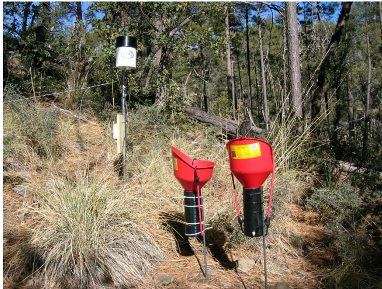
Figure 8. Rain Gauge (OR1) and bulk precipitation samplers at the lower field site at Oracle Ridge.
