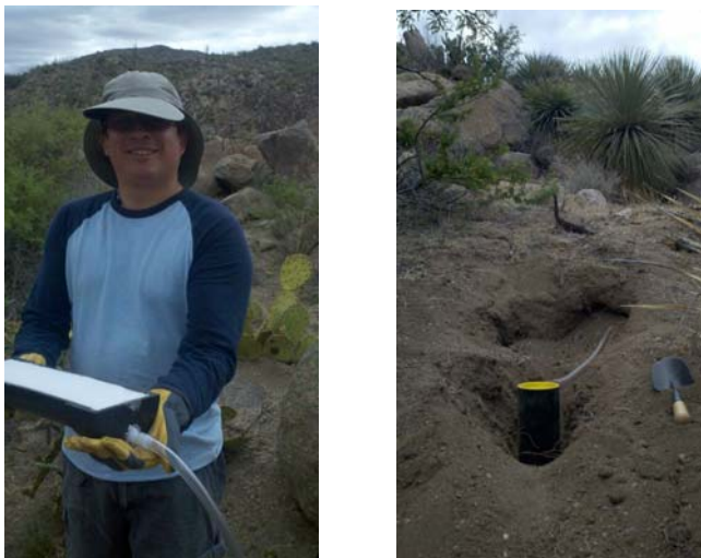
Figure 10. Zero tension soil solution samplers were designed following the procedure outlined by Dr. Eve Hinckley at the Boulder Creek CZO, and installed in the B2 desert site, where infrequent precipitation events and rapid water drainage from sandy soils precludes the use of slow sampling tension samplers.
