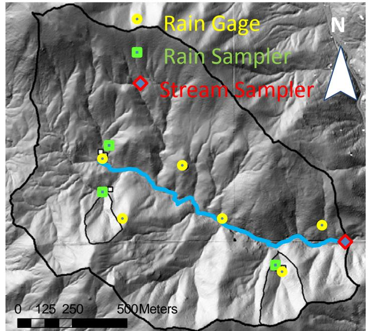
**Instrumentation.** In Marshall Gulch field equipment is being deployed in zero-order basins to measure water, carbon and energy stores and fluxes across the critical zone. Instrumentation includes rain gages, rain water samplers, streamflow flumes, snow melt lysimeters, shallow groundwater piezometers, soil moisture and soil temperature probes, soil water tensiometers, and soil water solution samplers.
