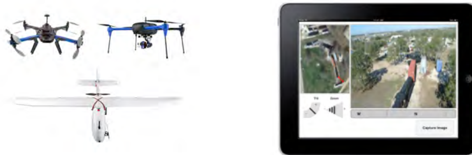
Figure 1. Small unmanned aerial vehicles available from Dr. Joshua Peschel's research group (left). On the right is an interface developed by Peschel (2012a) on a tablet allowing untrained users to use the UAVs.
