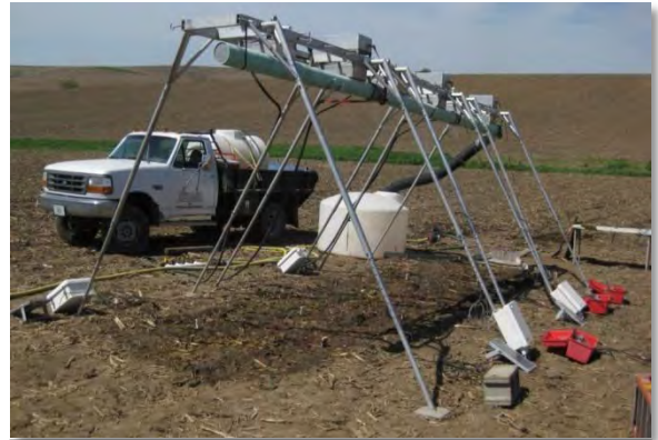
Figure 1: Rainfall simulator used to quantify enrichment ratios.
