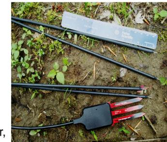
Soil Moisture/Temperature Probe (Decagon) Redox Sensors
