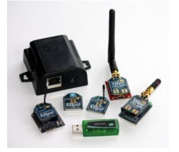
Xbee radio modules in the same network can use different power levels and configurations.
