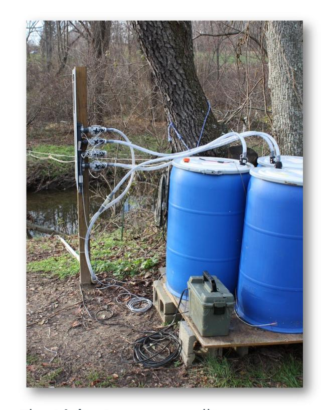
The **Dial-a-Pump** controller operates a bank of large solenoid valves that can fill multiple barrels for sampling the stream water during different parts of a storm.
