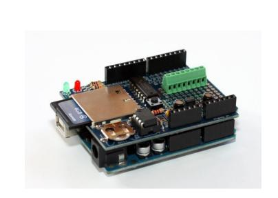
An interface board with memory card and clock creates a basic datalogger.
