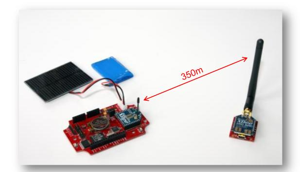
A solar powered logger with Xbee has a range of 350m to the base station, or 100m between logger nodes.
