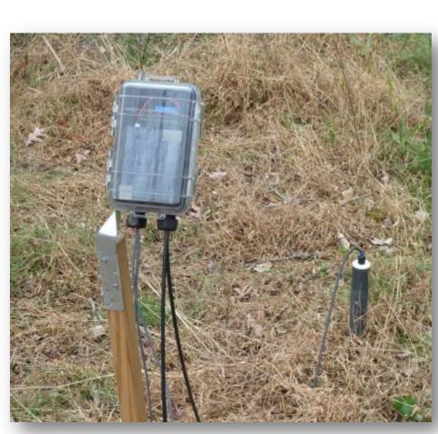
Solar powered well depth logger
