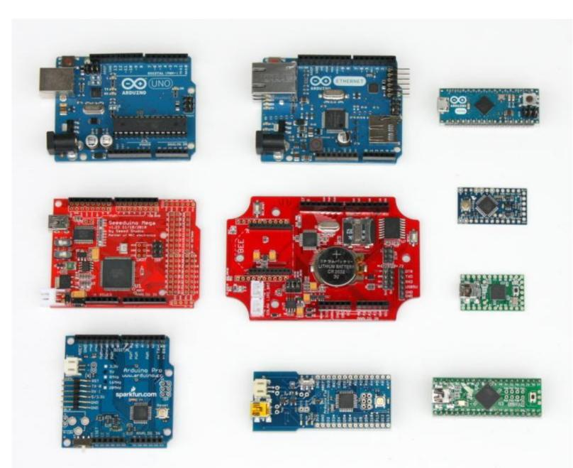
Arduino boards are available in a variety of sizes and configurations. Some have additional features like Xbee radio sockets, Ethernet ports and memory card slots. All of the boards shown here contain the same type of processor and are programmed the same, but the smaller boards are easier to fit into finished projects. Our dataloggers use a custom sensor interface board to easily connect various devices to the main board.
