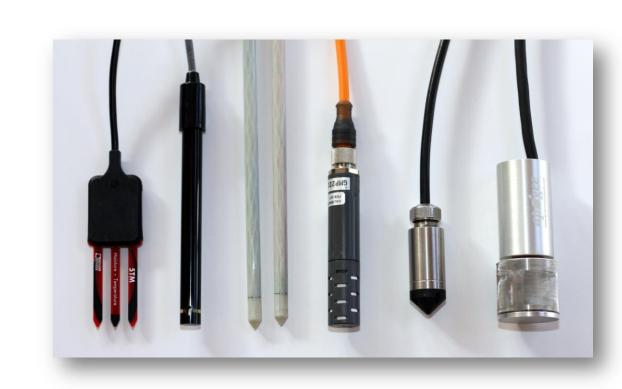
Some of the commercial sensors that can easily connect to Arduino loggers: soil moisture, conductivity, redox, CO<sub>2</sub> probes, pressure transducers, and oxygen sensors.
