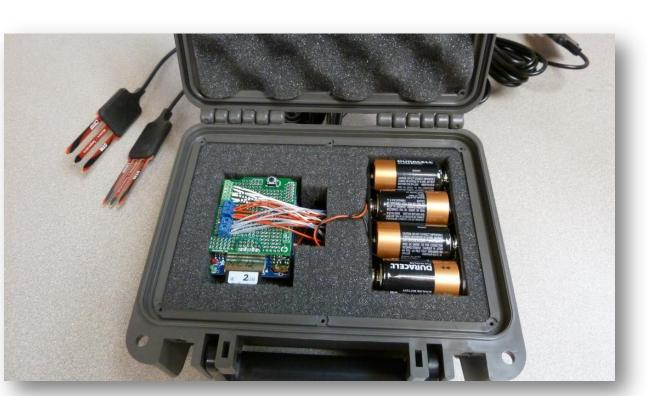
6-channel soil moisture probe logger
