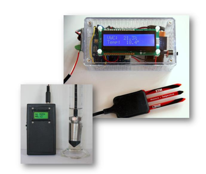
**Pressure Transducer Readout & Portable Soil Moisture Probe Tester**
