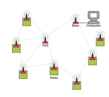
The Xbee radios form a selfhealing mesh network to transmit the data back to the coordinator.
