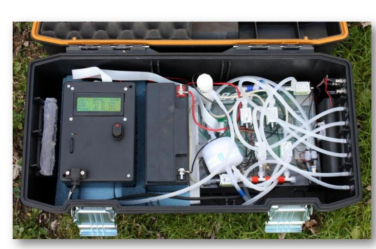
**Portable 3-chamber Soil Respirometer**
