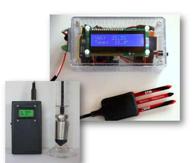
**Pressure Transducer Readout** & **Portable Soil Moisture Probe Tester** Useful for testing probes during deployment.
