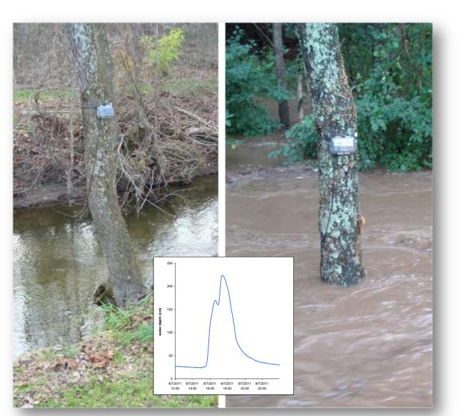
**Radio Reporting Stream Gage** An Arduino logger with Xbee radio sends live stream depth data to a base station that posts it to a web page.
