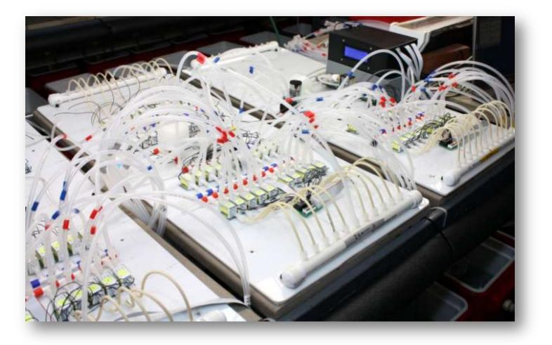
60-chamber Respirometer Controller Similar to the portable respirometer unit, this Arduino logger controls a LI-COR analyzer, pumps, and 120 separate solenoid valves that sample the rate of respiration in 60 jars of soil samples.
