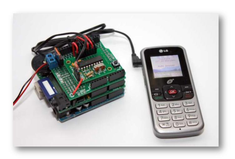
Remote Streamwater Sampling System (Also known as Dial-a-Pump) Researchers can remotely trigger a pump by calling the prepaid phone and then following the interactive voice menus to select pump options and hear live sensor value readouts.
