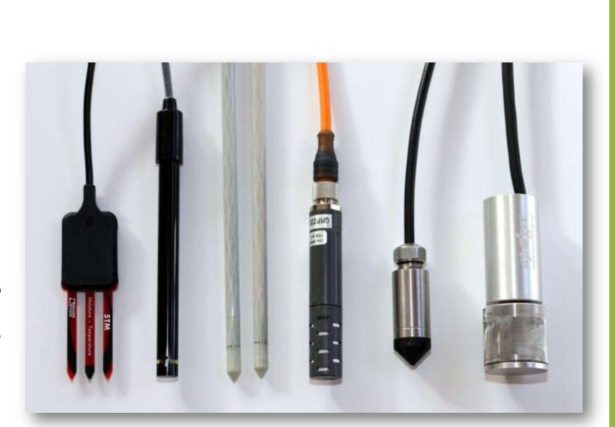
Some of the commercial sensors that can easily connect to Arduino loggers: soil moisture, conductivity, redox, CO<sub>2</sub> probes, pressure transducers, and oxygen sensors. These are the same sensors used with commercial dataloggers, so we can collect the same highquality data with our custom loggers.
