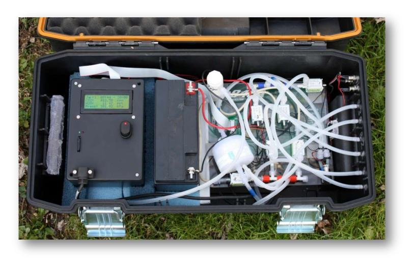
**Portable 3-chamber Soil Respirometer** The Arduino circuit displays live data from a LI-COR CO<sub>2</sub> analyzer, logs the data to a memory card, and operates solenoid valves and pumps to control the flow of air through custom respiration chambers.
