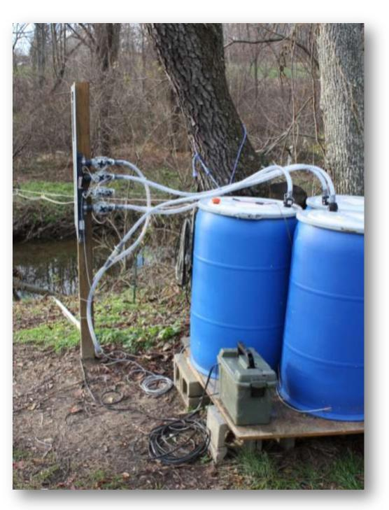
The **Dial-a-Pump** controller operates a bank of large solenoid valves in order to fill multiple barrels for sampling the stream water during different parts of a storm.
