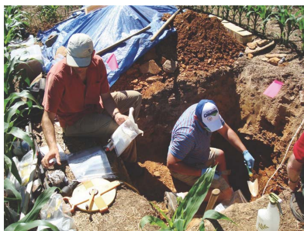
Fig. 17. Detailed pit sampling in 1.5 m agricultural soil pit.
