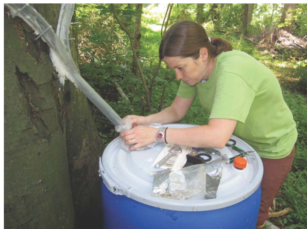
Fig. 15. Construction of stem-flow collection system.
