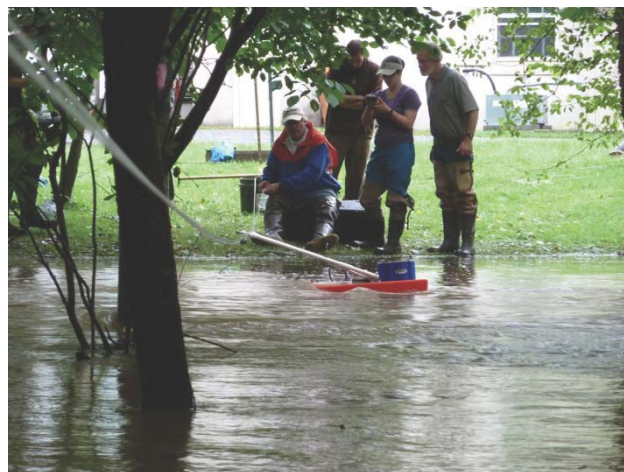
Fig. 16. One of 30 ADCP cross-section measurements of current and discharge measured at WCC-SWRC during Tropical Storm Lee.
