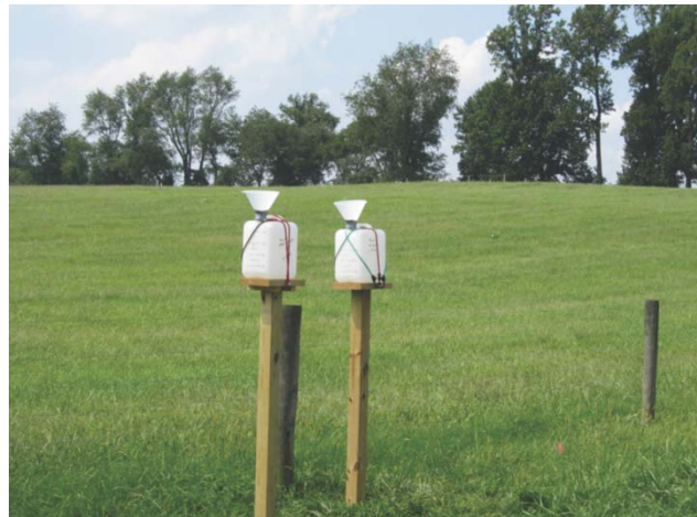
Fig. 14. Precipitation samplers for cosmogenic isotope samples.
