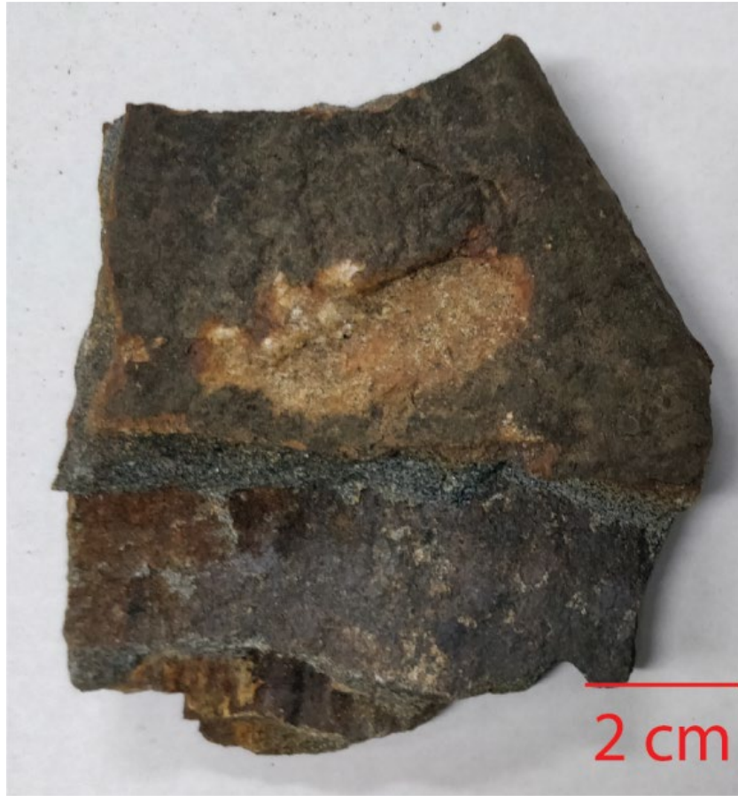
Figure 8: Meta-tonalite (BR04) in hand sample. Oxidation rinds were typical with this lithology. Despite a very fine grain size, cleavage plains of amphiboles and pyroxene were observable.
