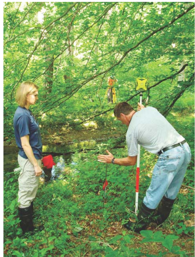
Fig. 9. Mapping a floodplain gravel layer prior to installing piezometer transect.
