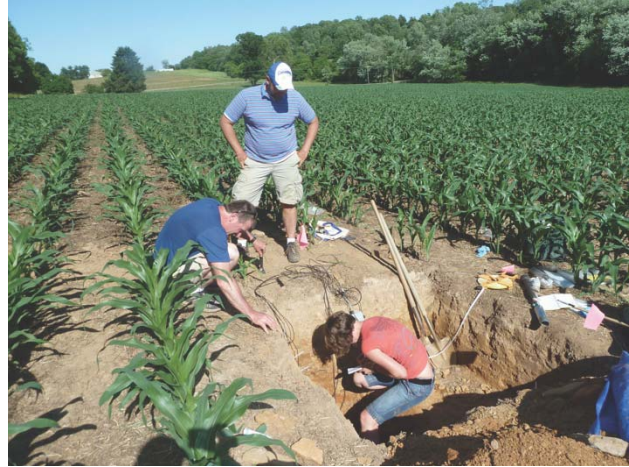
Fig. 10. Installation of redox and soil moisture/temperature probes in upland soil pit.
