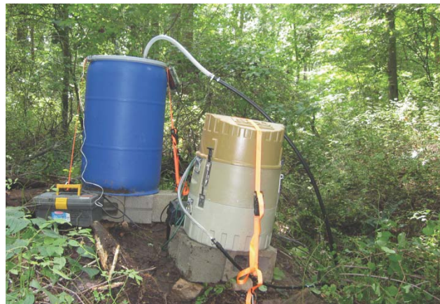
Fig. 11. Collection barrel with cell phone trigger attached (upper right) and ISCO sampler prepared for storm sampling.
