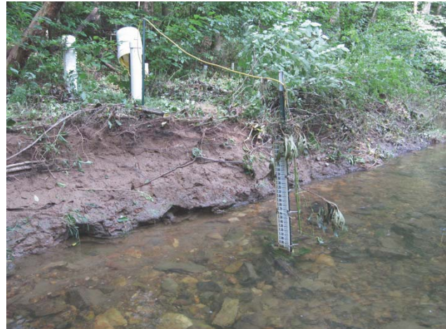
Fig. 8. Pressure transducer installation in 3 rd -order stream and riparian zone well.
