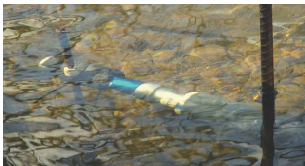
Fig. 6. Submersible diode-array spectrophotometer (s::can ® , spectro::lyser ® ) installed in 3 rd -order White Clay Creek.
