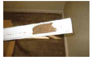
Figure 3. Placing material in the landslide chute.
