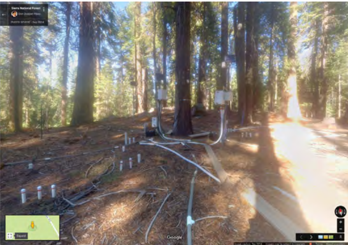
Figure 1. A CZ tree at the Southern Sierra Critical Zone Observatory. This is one of the most heavily instrumented trees in the world. PVC pipes in the ground allow access to equipment monitoring soil chemistry and temperature within the root system. Instruments embedded in the tree itself measure the flow of different fluids and monitor temperatures. The image is a screen-capture of a 360° interactive panorama captured using the Google Street View app. The panorama can be found at: https://goo.gl/maps/mHchVLBreVz .
