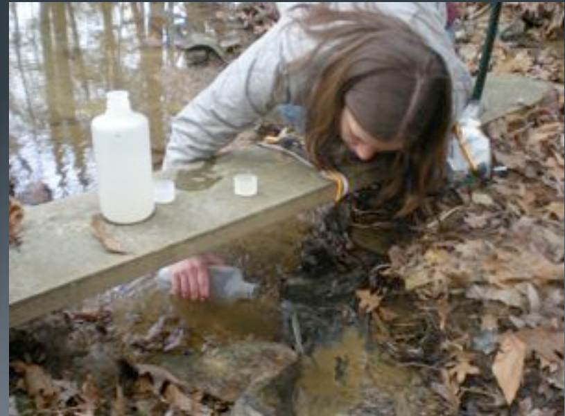
Water sampling at Christina CZO to measure suspended sediment composition
